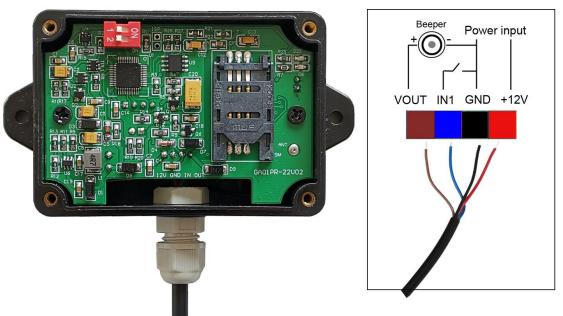
When IN1 input is shorted to GND, then will trigger the alarm
